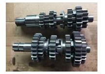
Check whether the gears of the main and countershaft assemblies have excessive or abnormal wear, and check whether the collars between the gears are deformed or fallen off.
