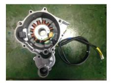
1. Install the magneto stator assembly to the left crankcase cover.
