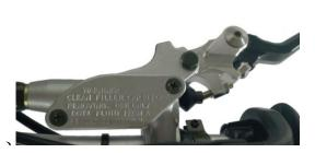
The brake fluid must be checked and replaced regularly. If the brake fluid is mixed with water, soil or other particles, the brake fluid should also be replaced.
