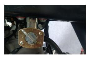
The K4 carburetor version adjusts the fuel supply through the fuel tank switch, which is located at the bottom of the left side of the fuel tank. By rotating the switch, you can control whether the fuel enters the carburetor, so as to achieve the control effect.
