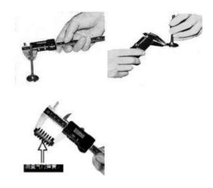
Check whether the valve is bent or the valve stem is abnormally worn, and measure the outer diameter of the valve stem. Repair limit value: Air intake: φ5.45mm Exhaust: φ5.43mm
