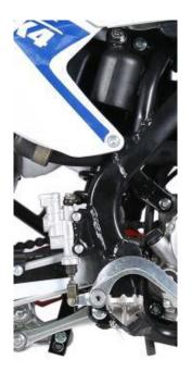
Check the rear shock absorber whether the airbag is normal and the spring is cracked or not,etc. If necessary, replace the rear shock absorber.
