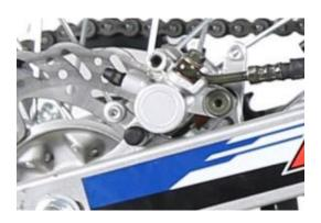
The rear wheel brake adopts a floating caliper disc brake, whose caliper body is located on the right side of the rear wheel and is fixed by a disc brake bracket.
