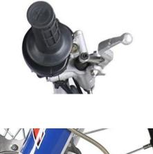
The front disc brake is controlled by the brake lever. Which located at the right end of the handlebar, and operated by the right hand.
