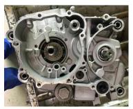
1. Install the positioning pin into the corresponding hole of the left box;
