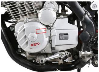
The engine number of the K4 is located on the inside of the engine gearshift lever
