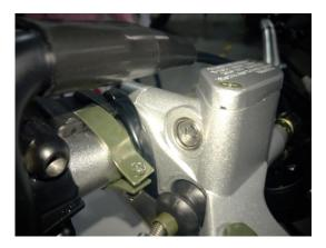
K4 model use hydraulic disc brakes, and the brake fluid level of the disc brakes can be checked through the observation hole.
