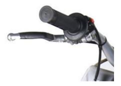
The clutch is controlled by the clutch lever, which located at the left end of the handlebar, and operated by the left hand.
