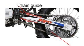
Check the wear of the chain guide and the chain protector on the swingarm. Under normal circumstances, these two can play a role in guiding the movement of the chain. If the wear is too large, it is not conducive to the normal movement of the chain and affects its transmission effect. Therefore, the excessively worn chain guide and Chain protector chain protector should be replaced in time to ensure that the motorcycle works normally.
