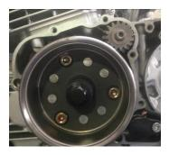
1. Install the double gear washer on the end face of the double gear;
