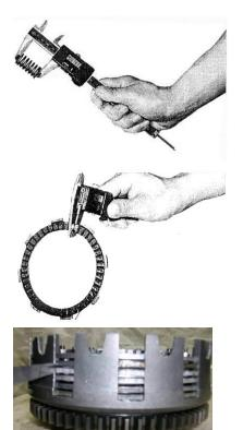
Measure the free length of the clutch spring Maintenance limit: 32.3mm
