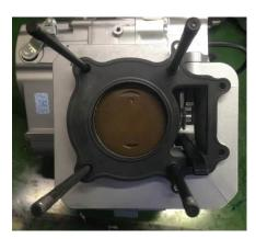
1. Install cylinder block positioning pins and new cylinder block gaskets;
