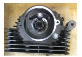
Inspection of valves and valve springs
