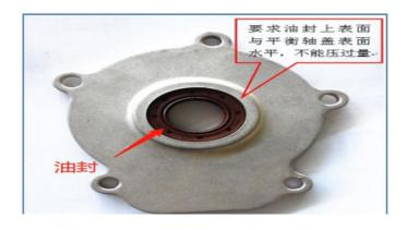
Remove the balance cover oil seal
