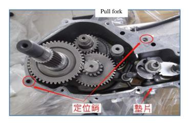
Install positioning pins (2) and new gaskets.
