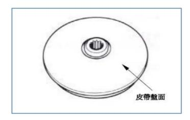
Install the sliding drive plate assembly on the crankshaft.
