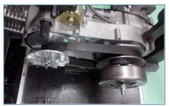
Assemble the clutch that has been installed in the drive belt on the drive axle.
