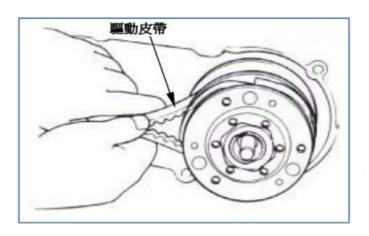
Squeeze the drive belt into the groove of the drive pulley as shown in the figure to loosen it, and then take out the belt and clutch at the same time. Remove
