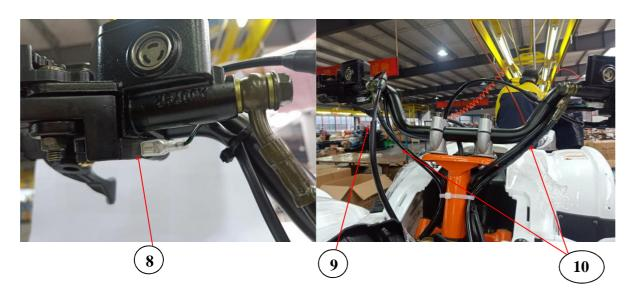
8. Brake sensor (one for left and right) 9. Throttle cable 10. Brake oil pipe
