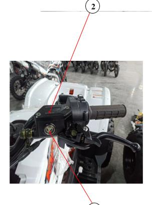
safe position; check whether the oil circuit and connection points are damaged, and if there is any damage, please replace it in time; check whether the main pump/caliper is damaged, and if there is any damage, please replace it in time.
