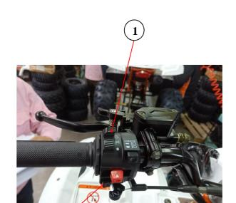
Turn the headlight switch 1 forward to the first gear, and observe whether the front fog lamp is on. If it does not, please check whether the line connector is loose or falling off. If the wiring is normal, replace the antifog lamp in time; In the second gear, observe whether the front headlights are on. If not, please check whether the line connectors are loose or fall off. If the wiring is normal, please replace the headlights in time.
