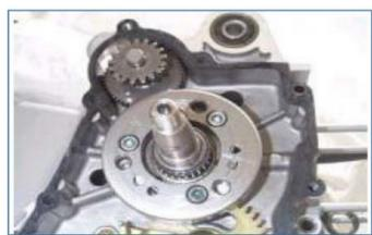
Install the starting driven gear on the starting clutch.
