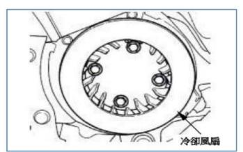
Remove the cooling fan (bolt X4)
