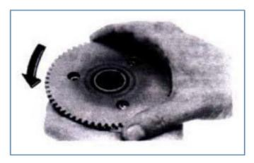
Fix the starting clutch and rotate the starting driven gear.
