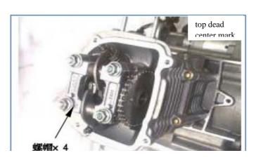
Remove the camshaft fixing seat and rocker arm group.
