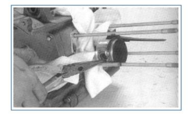
Push out the piston tip from the end of the buckle.
