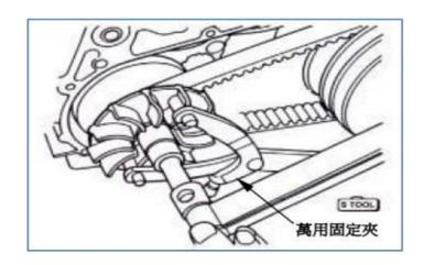
Use the universal fixing clip to fix the clutch cover, and remove the nut and clutch cover.
