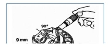
Measure the outer diameter of the piston.
