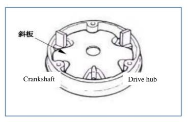
Remove the inclined plate.
