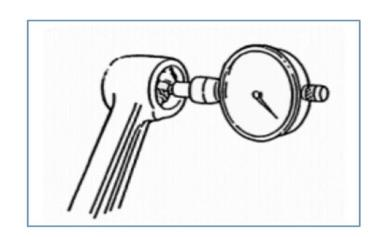
Measure the inner diameter of the piston pin hole.
