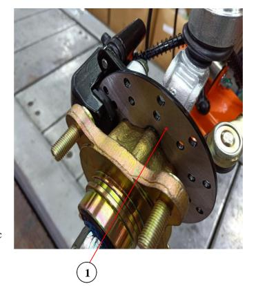
Check the mini. thickness of brake lining 2.
