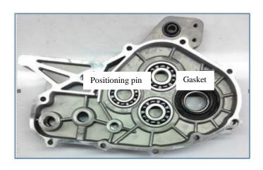
Coat the lip of oil seal of drive shaft, wheel output shaft and gear shaft with butter, install
