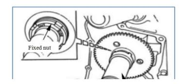
Apply engine oil to the threads of the fixed nut.
