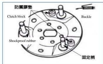
Spread a little butter on the fixed pin, but there should be no butter on the clutch block. If there is butter on the clutch block, replace it.
