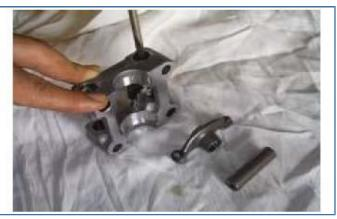
Measure the inner diameter of the valve rocker shaft hole of the camshaft fixing seat.
