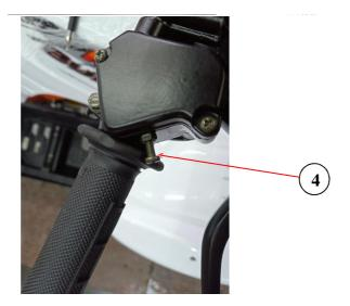
Pinch the brake lever with your hand and observe the tail light. If the tail light does not light up, please check whether the line connector is loose or fall off. If the wiring is normal, replace the tail light in time.
