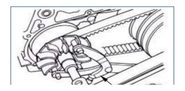
Install the drive plate, washer and nut.
