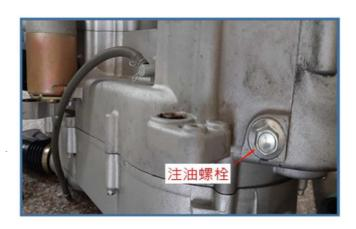
Remove the gear oil injection port bolt, place a measuring cup under the drain bolt, remove the gear oil drain bolt, introduce the gear oil into the measuring cup, and check whether the gear box oil meets the standard value. If the amount of oil is too low, add gear oil.
