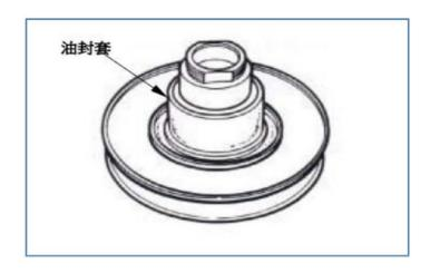
Install the oil seal sleeve.
