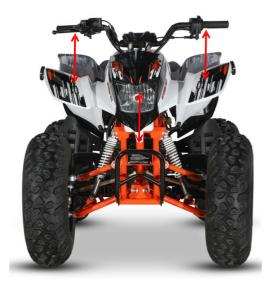
Place the car in a horizontal position and slowly turn the direction handle to the left and right to confirm whether it can turn smoothly and flexibly. If there is obstruction in some places, check whether the main cable assembly and cables interfere. If the end Position of the steering pull rod is not observed, confirm whether there is interference and whether the steering bearing is damaged.
