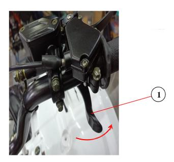
Check the free stroke of throttle button 1
