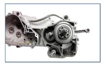
Turn the left crankcase down and disassemble the right crankcase. Separate the left/right crankcase.
