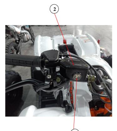
and right, and then remove the oil cup cover after the brake pump assembly is in a horizontal state.
