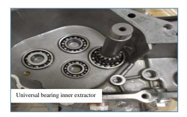
Install a new drive shaft bearing on the gear box.
