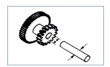
Measure the outer diameter of starting idler gear shaft.
