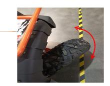
Remove the front wheel when there is shaking, and check the wheel hub
