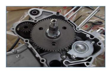
Use a universal holder to fix the starting driven gear.
