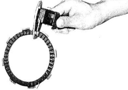
Check if there is any distortion on the surface of the clutch follower, check with the feeler gauge.
