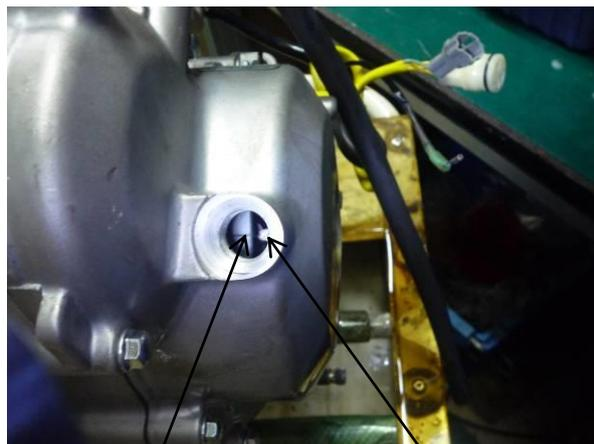
NC250 Magneto rotor timing mark
