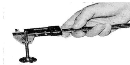
Contact surface width maintenance limit value: 1.5mm
