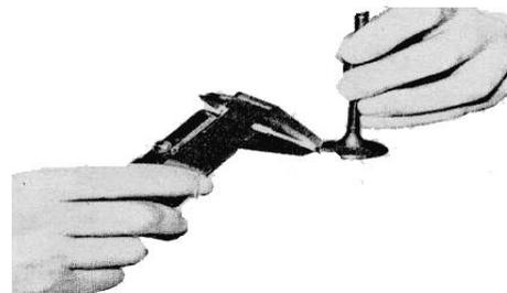
Measure the free length of the valve spring: 48.35mm
