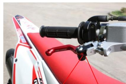
**Danger:** please test the braking system (including front brake and rear brake) before each start. If you feel soft when pinching the brake handle or pressing the brake pedal, there may be air in the corresponding pump or oil circuit, or one or more parts of the corresponding braking system are not in good condition. In case of any of the above, please check the brake system and contact the KAYO dealer immediately.
